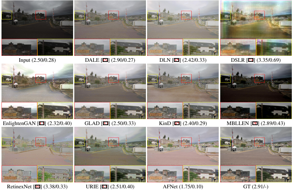
Figure 5: Performance of SoTA algorithms on moderately dark image from SICE dataset captured at -1ev setting. Numbers in brackets represent NIQE and LPIPS score respectively.
