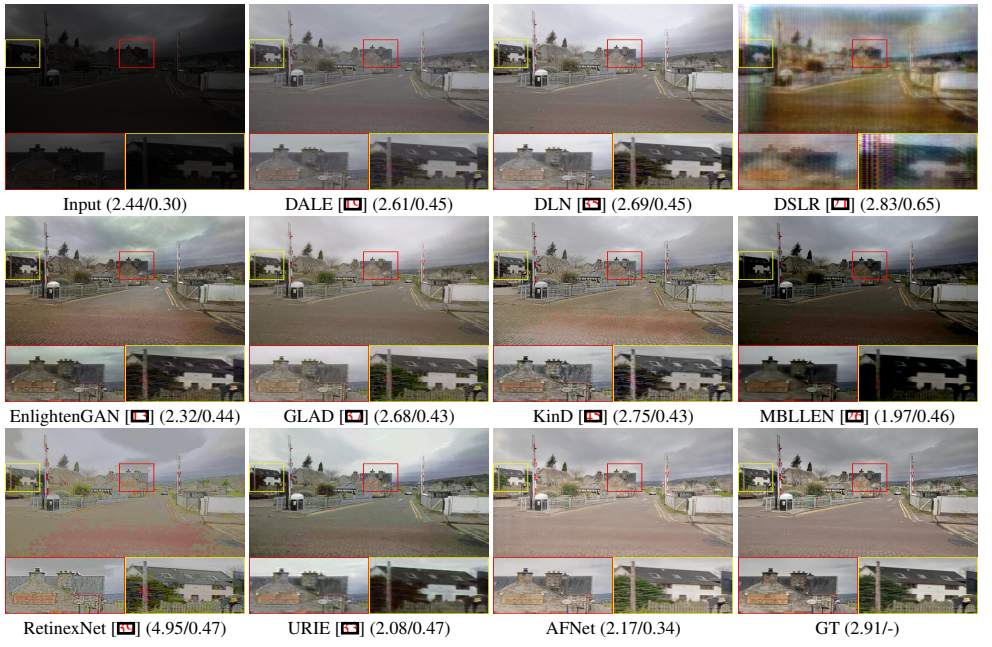
Figure 4: Performance of SoTA algorithms on extremely dark image from SICE dataset captured at -3ev setting. Numbers in brackets represent NIQE and LPIPS score respectively.
