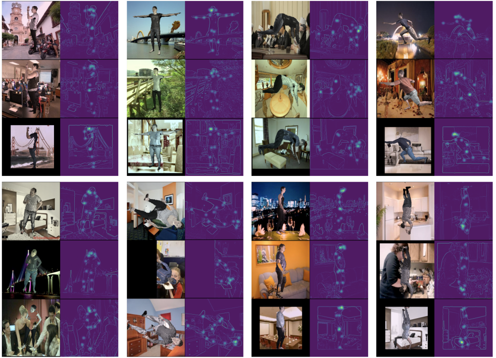
Figure 7: Examples of synthetic RGB training images and corresponding edge-image + 2D joint heatmap proxy representations. Images within each group of 3 use the same pose (selected from common 3D SMPL pose datasets [5, 10, 19]) but different random body shapes, clothing textures, backgrounds and lighting parameters. The synthetic RGB images are computationally cheap and far from photorealistic - however, edge-filtering significantly reduces the synthetic-to-real domain gap.
