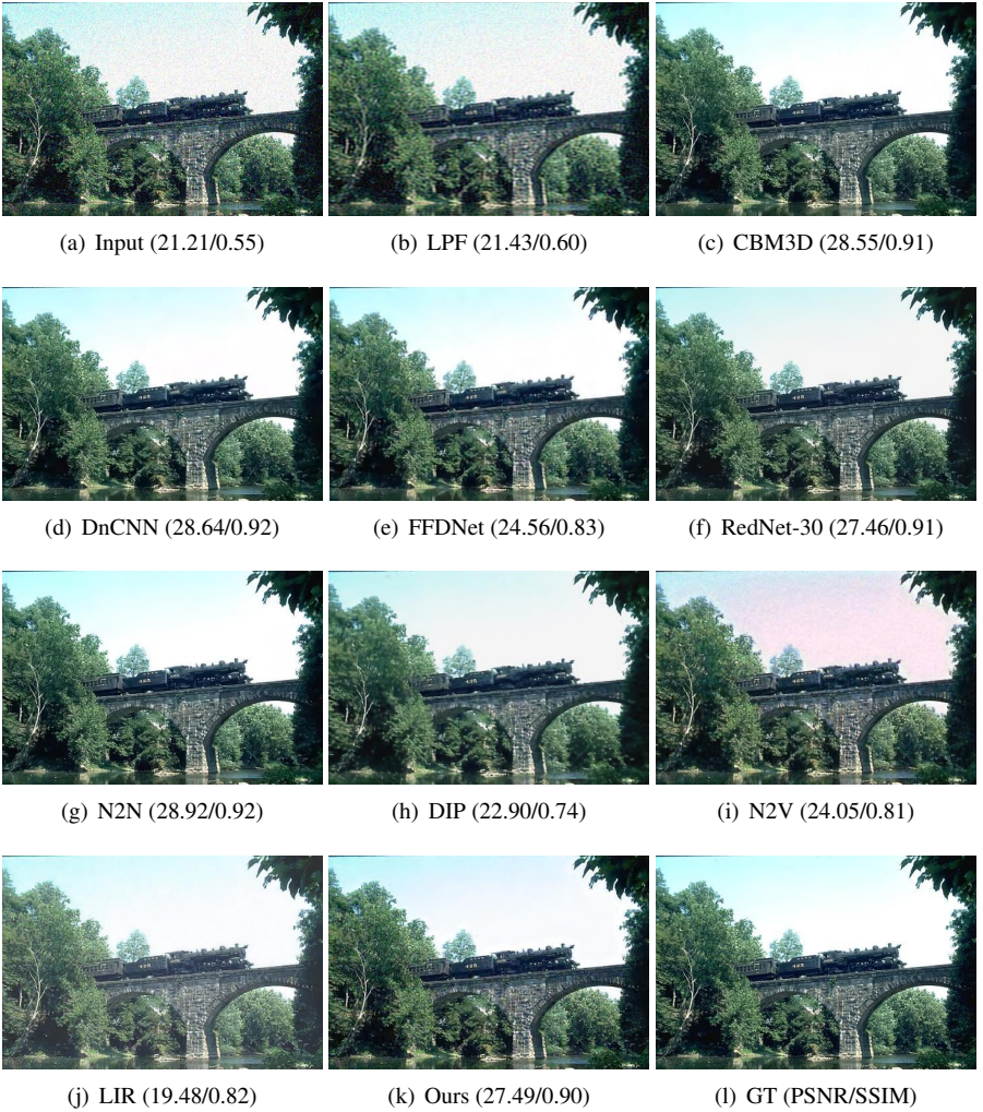
Figure 6: Qualitative results of our method and other baselines on CBSD68 corrupted by AWGN with a noise level \sigma = 25 .
