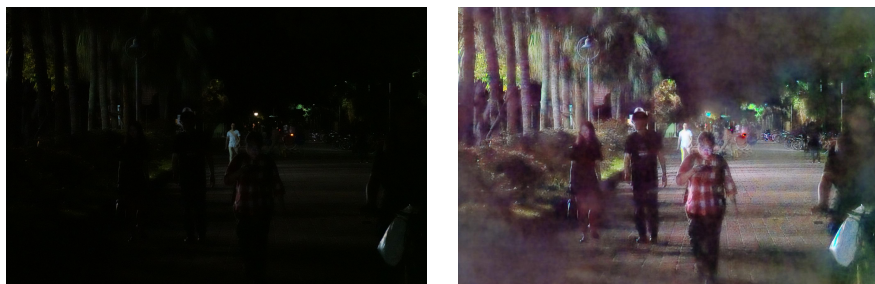
Figure 10: Left: input image. Right: intermediate representation enhanced by the proposed image enhancement module.
