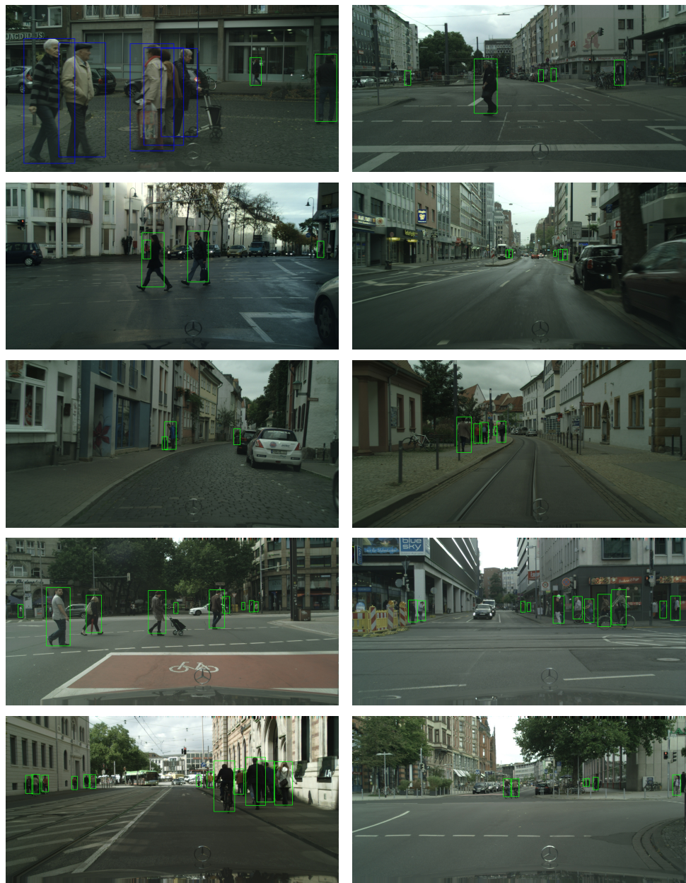
Figure 6: Examples for pseudo-labels (green boxes) if only the largest 1% of pedestrians are annotated (blue boxes). Although only very few, extremely large pedestrians are labeled, correct pseudo-labels are created for a substantial part of missing annotations.
