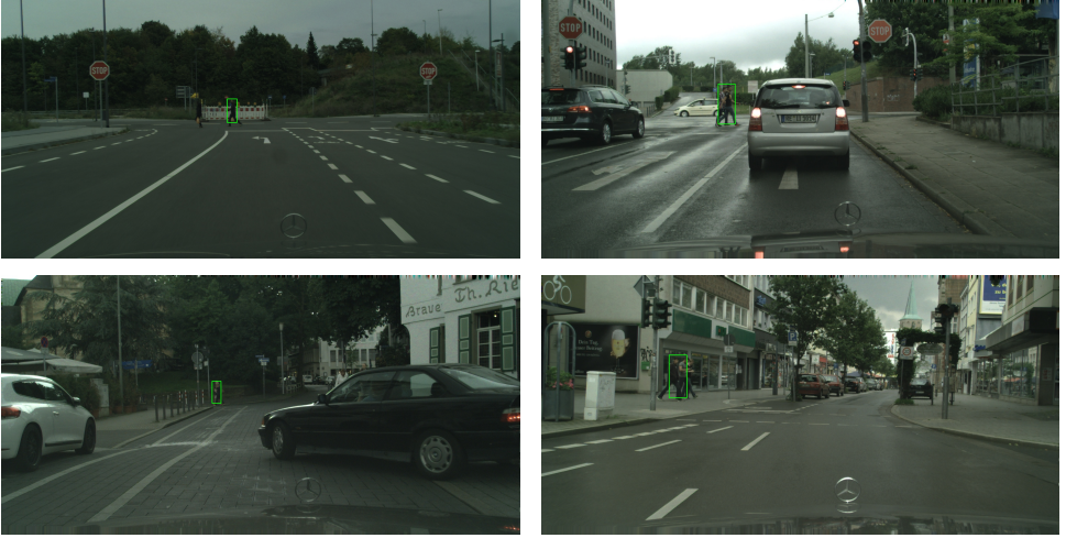
Figure 7: Failure cases for pseudo-labels (green boxes) if only the largest 1% of pedestrians are annotated (blue boxes).
