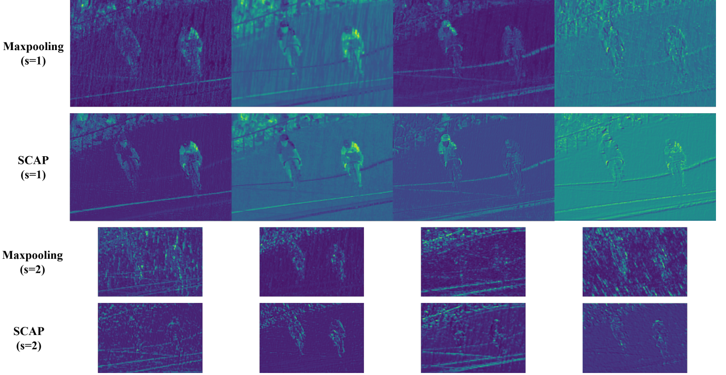
Figure 2: The visualized feature maps with the proposed SCAP and the conventional MaxPooling layers for another image.
