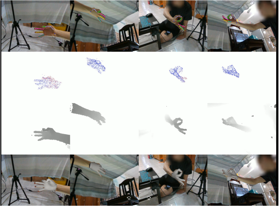
Figure 1: Sequence sample from our proposed MVHand dataset. From top to bottom: RGB images with 2D poses, point cloud ground truth, depth maps and mesh images, respectively. Please go to see our dataset video for more details.
