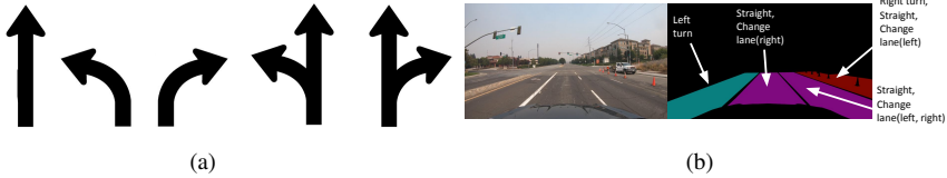
Figure 9: Subplot (a) shows the 5 different Symbolic Road Marking attributes annotated in the the EPOSH dataset dataset - Straight, Left, Right, Straight-Left & Straight-Right. All other SRMs are annotated as ‘other’. Subplot (b) shows an example of affordance annotations from the EPOSH dataset.
