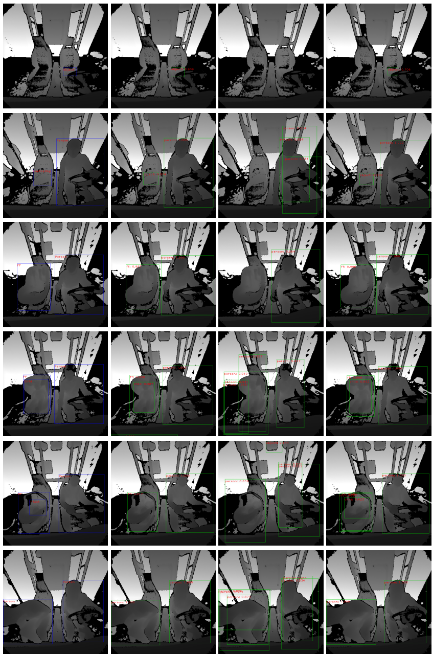
Figure 5: Depth images showing boxes predicted by Faster R-CNN when trained on depth images from train_real , train_syn and finetuned on train_real imagesets.
