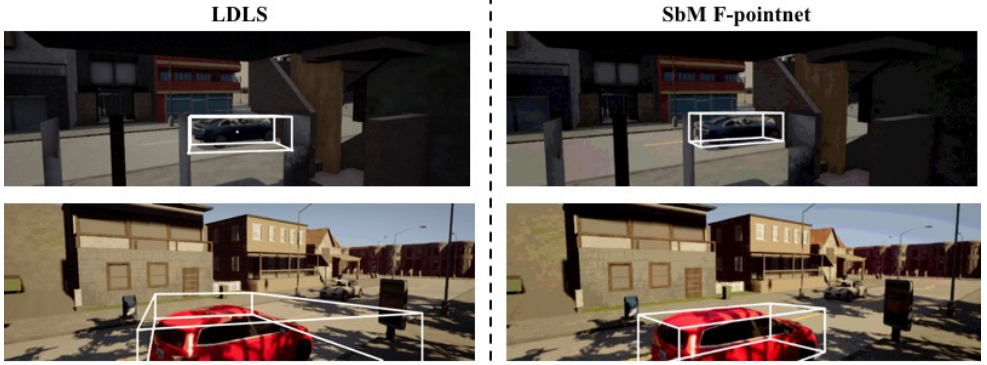
Figure 2: Visualizations of 3D object detection. We show paired examples of the results of LDLS [1] (left) and SbM-trained frustum PointNet (ours, right) on the CARLA test set. While LDLS estimates the bounding box roughly, the SbM-trained frustum PointNet is able to obtain much tighter and better-oriented boxes.
