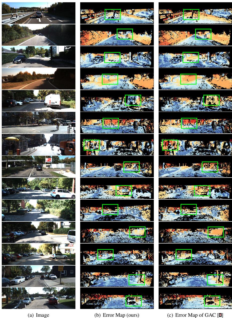
Figure 3: Qualitative comparison to GAC [9] on the validation set of KITTI single-image depth prediction benchmark.
