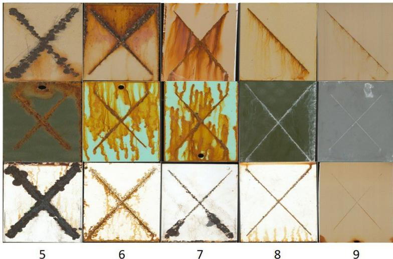
Figure 1: Three sample images per corrosion rating class 5 - 9 from our data set.
