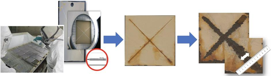
Figure 2: Material experimentation and corrosion rating process. *Left*: Application of coatings to test panels. Test panels are coated with a pretreatment, primer, and topcoat and then scribed with tungsten carbide (circled in red). *Middle*: Panel is placed in accelerated corrosion chamber to initiate corrosion. *Right*: Final time point. Corrosion width is measured at 12 evenly distributed locations along the scribes and assigned an appropriate rating.
