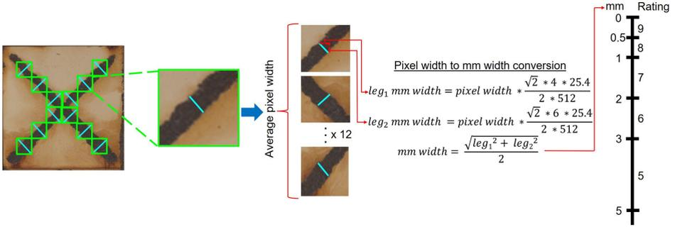
Figure 4: Non-expert rating procedure. Corrosion areas are identified in 12 locations on an image, measured on the computer in a pixel width, averaged across the 12 boxes, converted to a mm width, and then assigned the appropriate scribe corrosion rating 0-10.
