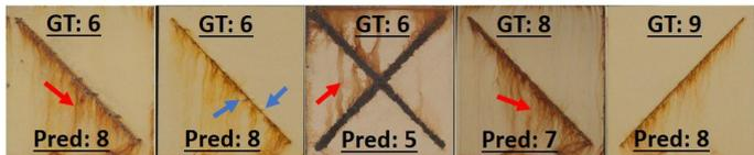
Figure 6: *Misclassified* samples with ground truth (GT) and predicted (Pred) ratings noted. Red arrows identify water stain, blue arrows identify raised blistering under the topcoat.
