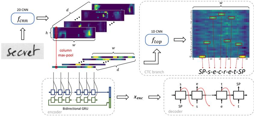
Figure 1: Proposed architecture. The word image is processed through a 2D convolutional backbone, leading to  $w \times d$ -sized feature map. The model then branches to two components, a CTC branch and a Seq2Seq (encoder/decoder) branch, combined through a multi-task loss.
