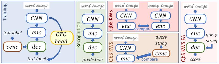
Figure 2: Overview of the different setups of the proposed system. Evaluation can be categorized to recognition and three spotting cases: QbE, QbS and QbS by force-alignment (FA).
