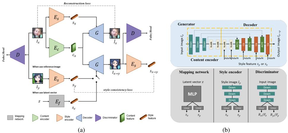
Figure 3: (a) Overview of proposed model. (b) Architecture of content encoder, style encoder, mapping network, decoder and discriminator.
