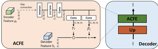
Figure 2: In the adaptive content feature enhancement (ACFE) block, the encoder feature  $g_i$  is first projected onto an embedding space with only one channel. And then increase the channel of feature by convolution. Finally, convolved to produce the modulation parameters  $(\gamma_i, \beta_i)$ . These parameters are element-wise multiplied and added to the decoder feature  $h_i$ .
