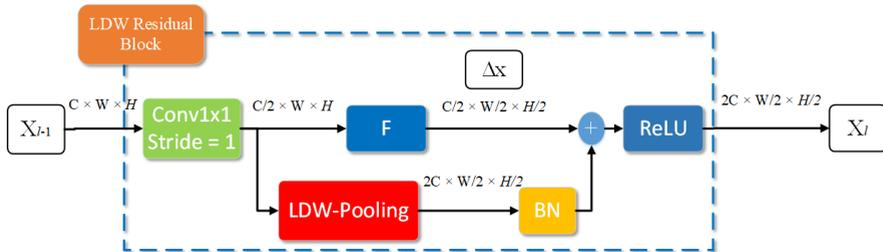
Figure 4: **LDW-Pooling in Bottleneck.** With LDW-Pooling on  $X_{t-1}$  at residual branch. We slightly change the output of  $Conv1 \times 1$  with the channel number equal to the input channel. This makes the output channel of LDW-Pooling correspond to the original output.
