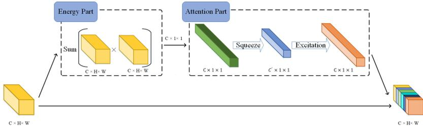
Figure 2: The **energy attention mechanism** for feature enhancement consists of two parts. The “Energy” part calculates feature energy in each channel as the sum of squared feature values. The “Attention” part learns which channel is important via squeeze-and-excitation [6].
