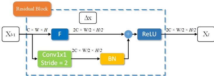
Figure 3: **Original Bottleneck.** *BN* and *ReLU* denote to batch normalize and ReLU function. With several convolutions to extract the feature to get  $\Delta x$ . The residual branch simply get features from  $X_{t-1}$  with  $1 \times 1$  convolution with 2-stride if needed.
