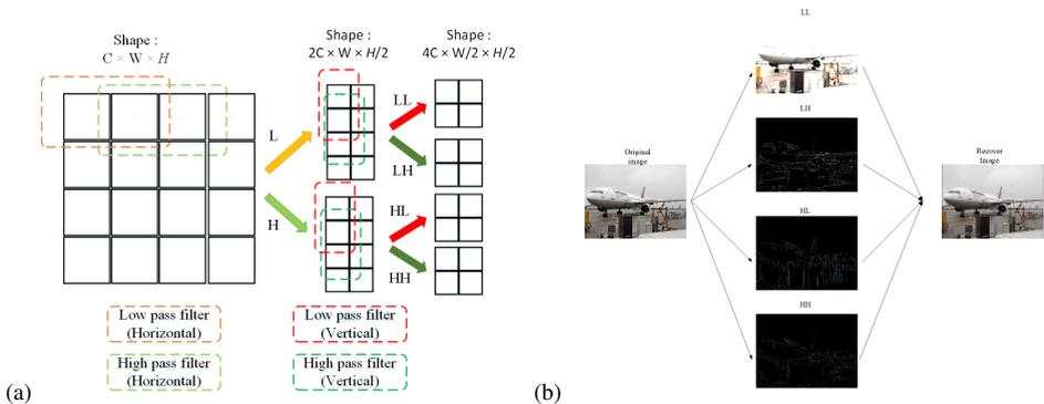
Figure 1: **Overview of the proposed LDW-Pooling method.** (a) Given an input signal of  $C$  channels of width  $W \times$  height  $H$ , we use high-pass (H) and low-pass (L) filters in the size of  $1 \times K$  (horizontally) and  $K \times 1$  (vertically) to decompose each 2D feature map into four subbands, LL, HL, LH, HH. (b) Reconstructed result after LDW-Pooling decomposition and recovering by UNet with PSNR=33.1.
