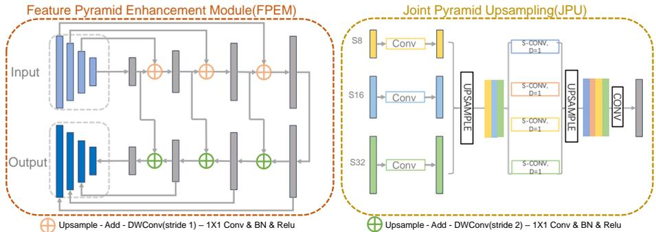
Figure 4: The architecture of FPEM [16] and JPU [18] module.
