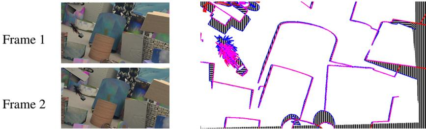
Figure 1: Ocs align with MBs in this FlyingThings3D [20] frame pair. Vertical stripes denote  $O_1$ , i.e., Ocs in frame 1. Horizontal stripes are direct-warps to frame 1 of Ocs in frame 2 ( $D(O_2)$ ), and checkerboard patterns are  $O_1 \cap D(O_2)$ . Red curves are  $M_1$  (similar notation for MBs  $M$  as for Ocs  $O$ ), blue ones are  $D(M_2)$ , and purple ones are  $M_1 \cap D(M_2)$ .
