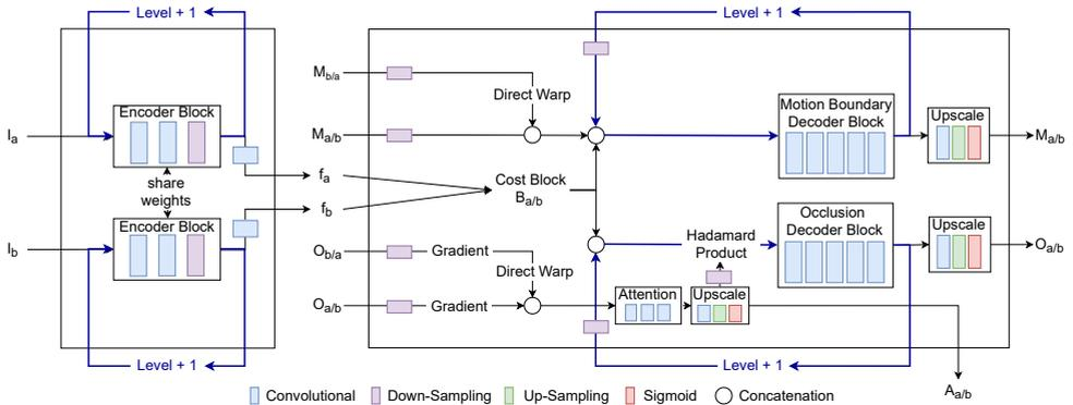
Figure 5: MONet predicts bidirectional  $M_{a/b}$  and  $O_{a/b}$  maps in each level  $l$  using bi-directional predictions ( $M_a, M_b, O_a, O_b$ ) and cost block ( $B_{a/b}$ ) from the previous level  $l - 1$ . Blue arrows represent the main flow of information across levels.
