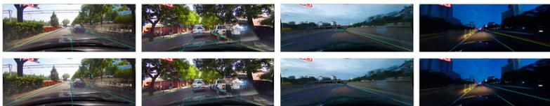
Figure 6: Visual results of ERFNet (upper) and our method (lower) on the CULane test set. Green lines: ground-truth; blue line: true-positive; and red lines: false-positive.
