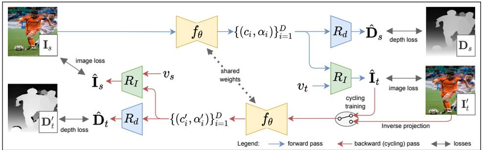
Figure 1: Proposed CycleMPI: a source image  $\mathbf{I}_s$  is fed into a neural network  $f_\theta$ , which produces an MPI representation w.r.t. the *source viewpoint*  $v_s$ . This MPI is then rendered in the target viewpoint  $v_t$ , resulting in  $\hat{\mathbf{I}}_t$ , which can be fed back into the network. The new MPI produced w.r.t. to the *target viewpoint* is then rendered in the source viewpoint, closing the loop for cyclic supervision. Depth maps are used as additional supervisions.
