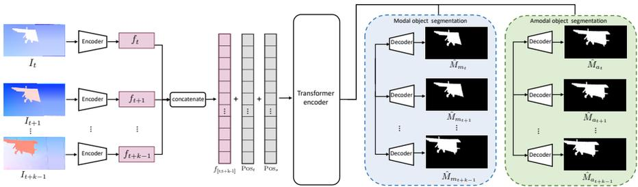
Figure 5: **Illustration of our proposed dual-head hybrid architecture for independent motion segmentation.** Our model takes a sequence of optical flows as input, and encodes each with a light-weight ConvNet, then positional spatio-temporal information is added to the outputted features  $f_{[t,t+k-1]}$  before passing through the transformer encoder. Lastly, the output is fed into the dual-head decoder, predicting amodal  $\hat{M}_{a_i}$  and modal masks  $\hat{M}_{m_i}$ .
